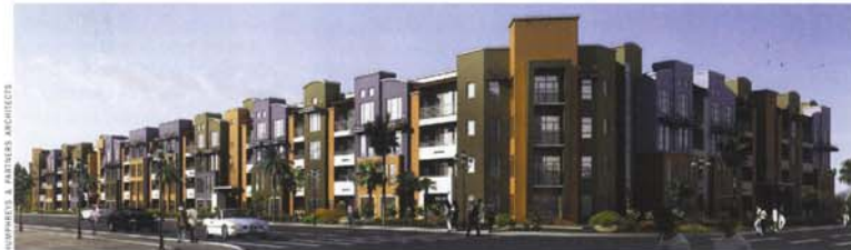
When using tunnel form construction, by crisscrossing forms and introducing curved walls, it is possible to make a building that looks like it is based on a column structure, rather than a load-bearing wall building.
