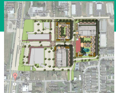
The site plan shows parking decks wrapped by the apartment buildings on all major exposures. The commercial footprints extend left toward McFarland Boulevard.
